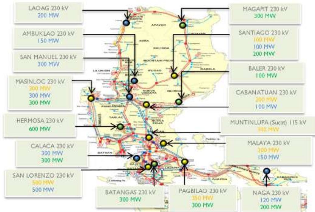
Figure 22: Locations where new power plants may connect without the need for any significant transmission reinforcement: yellow = 2011; blue = 2015; green = 2020
