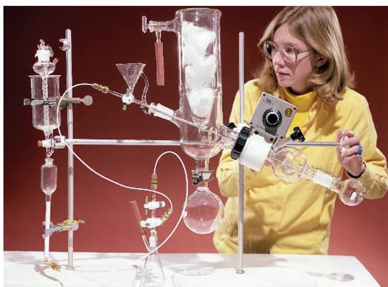
Fig. 12. Dr. Joanna S. Fowler and her [ 18 F] Fluorodeoxyglucose synthesis setup. Source: https://www.bnl.gov/newsroom/news.php?a=111461
