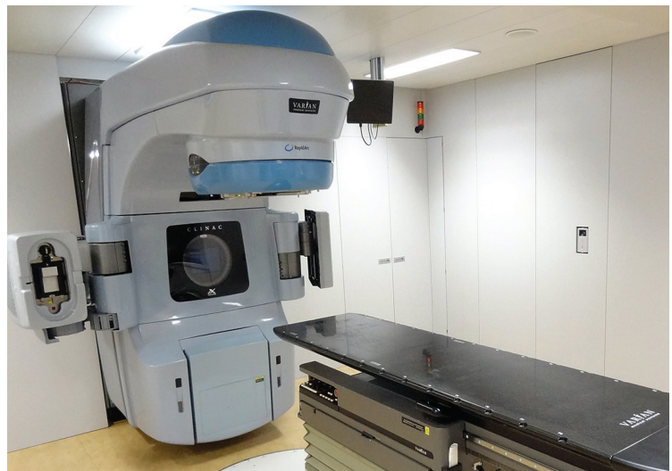
Fig. 5b. Linear accelerator machine Source: https://www.oncologysystems.com/blog/making-varian-linear-accelerator-vault-obi-board-imaging-ready
