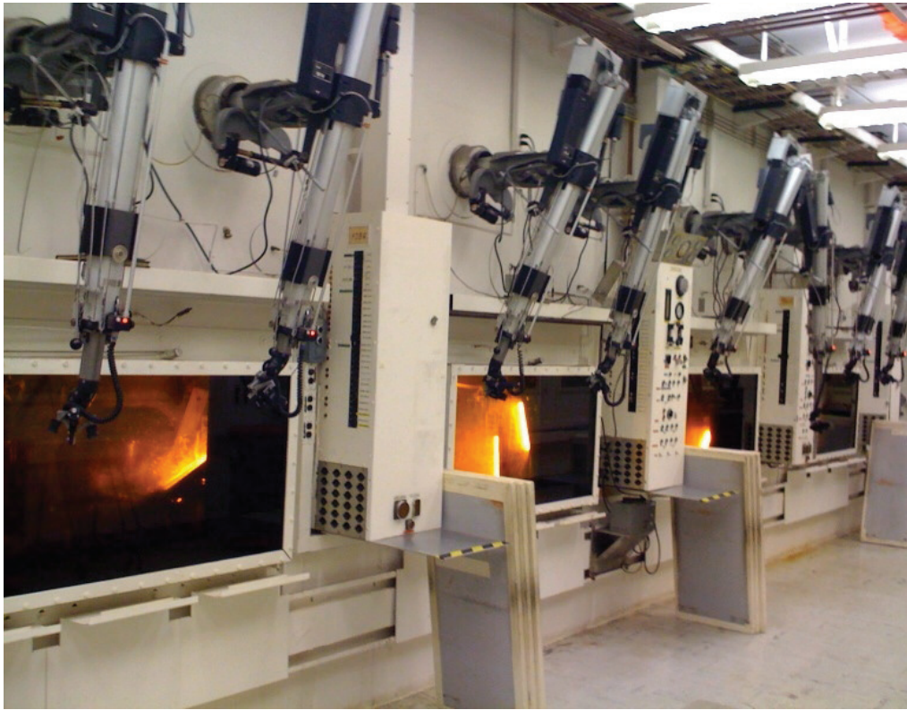
Fig. 15. Argonne National Laboratory research reactor hot cells.
