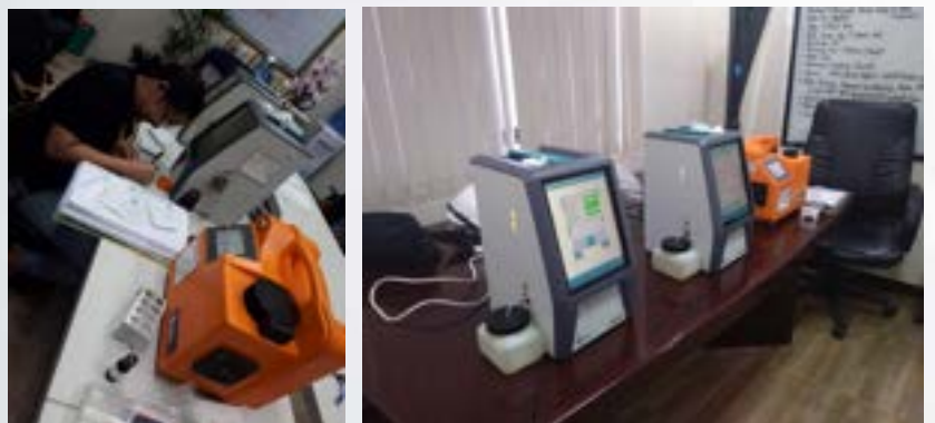
Figure 34. On site screening of petroleum samples using DOE's portable testing equipment
