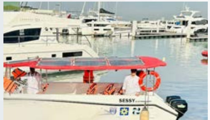
Figure 48. Safe, Efficient, and Sustainable Solar-Assisted Plug-In Electric Boat (SESSY E-Boat)
