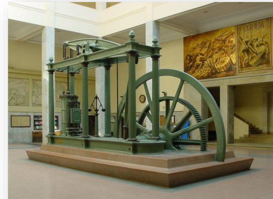
Watt steam engine used heavy flywheel to smooth output
