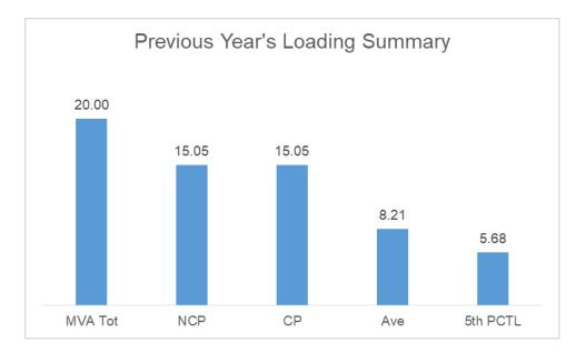
The Non-coincident Peak Demand is 15.05MW, which is around 75.25% of the total substation capacity of 20MVA at a power factor of 98.88%. The load factor or the ratio between the Average Load of 8.21MW and the Non-coincident Peak Demand is 54.55% of the Non-coincident Peak Demand. A safe estimate of the true minimum load is the fifth percentile load of 5MW which is 37.74% of the Non-coincident Peak Demand.
