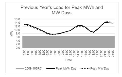
With majority of Residential Customer the off peak falls at 7 A.M. (7.4MW) each day and will rise again until it reaches 3 P.M. (12MW) being the peak load during day time. Then will descend again between 5 P.M. to 6 P.M. (8.6MW) and ascend to night time peak load (15.05MW) at 10 P.M.
