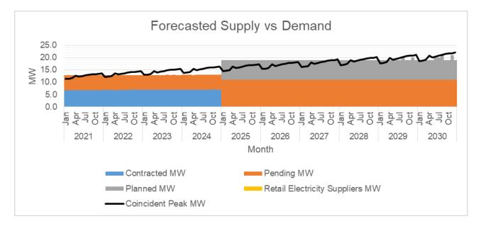
As illustrated above, the planned MW supply overlaps the projected Coincident Peak Demand. The reason is that there are indicative or potential spot loads that will connect to PRESCO.
