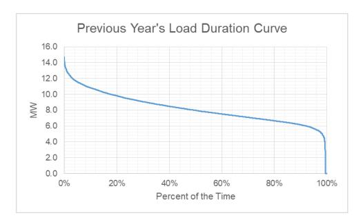
Based on the Load Duration Curve, the minimum load is 6MW and the maximum load is 15.05MW for the last historical year. This is because most consumers are residential where they consume most of the energy during night time. Also, due to the high number of connections also due to COVID-19 Lockdown almost every people are on their respective houses which resulted to higher electric consumption.
