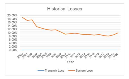
Historically, System Loss ranged from 18.89% to 8.16%. System Loss peaked at 18.89% on year 2000.
