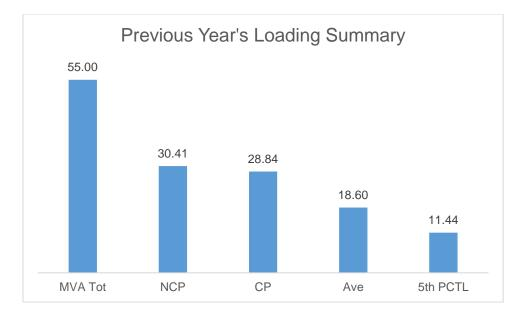
The Non-coincident Peak Demand is 30.41 MW, which is around 55.29% of the total substation capacity of 55 MVA at a power factor of 96.22%. The load factor or the ratio between the Average Load of 18.60 MW and the Non-coincident Peak Demand of 30.41 is 38.83%. A safe estimate of the true minimum load is the fifth percentile load of 11.44 MW which is 62.38% of the Non-coincident Peak Demand.
