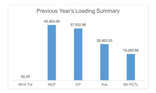
The Non-coincident Peak Demand is 40.46 MW, which is around 74% of the total substation capacity of 55 MVA at a power factor of 99.25%. The load factor or the ratio between the Average Load of 26.46 MW and the Non-coincident Peak Demand is 65%. A safe estimate of the true minimum load is the fifth percentile load of 19.28 MW which is 48% of the Non-coincident Peak Demand.
