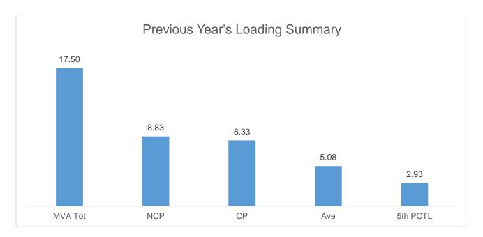
The Non-coincident Peak Demand is 8.83 MW, which is around 51 % of the total substation capacity of 17.5 MVA at a power factor of 98%. The load factor or the ratio between the Average Load of 5.08 MW and the Non-coincident Peak Demand is 57 %. A safe estimate of the true minimum load is the fifth percentile load of 2.93 MW which is 33 % of the Non-coincident Peak Demand.
