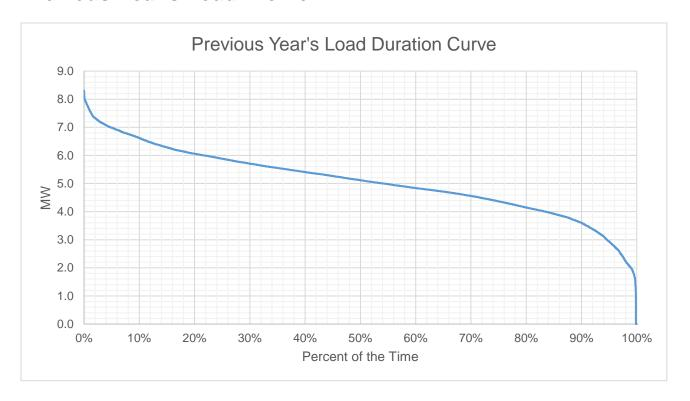
Based on the Load Duration Curve, the minimum load is 2.93 MW and the maximum load is 8.83 MW for the last historical year.
