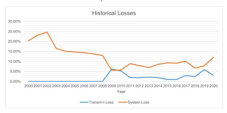
Historically, Transmission Loss ranged from 1.86% to 3.06% while System Loss ranged from 7.91% to 12%. Transmission Loss peaked at 5.88% on year 2019 because of the increase in MWH consumption. System Loss peaked at 12% on year 2020 because of immediate drop in energy consumption.
