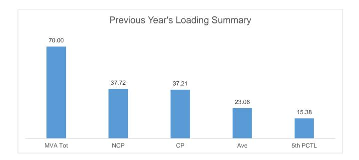
The Non-coincident Peak Demand is 37.75 MW, which is around 62% of the total substation capacity of 60 MVA at a power factor of 98%. The load factor or the ratio between the Average Load of 60 MW and the Non-coincident Peak Demand is 61.13% of. A safe estimate of the true minimum load is the fifth percentile load of 15.38 MW which is 40.77% of the Non-coincident Peak Demand.
