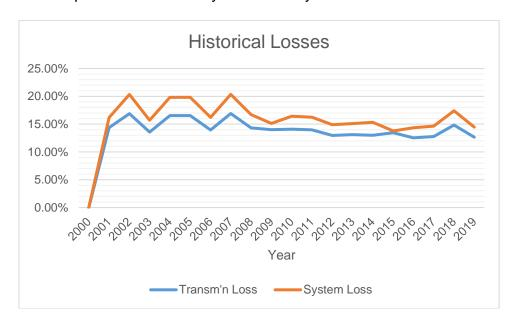
Historically, Transmission Loss ranged from 13.57% to 16.91% while System Loss ranged from 13.78% to 20.35%. Transmission Loss peaked at 16.91% on year 2008 because of sales was lower than the purchase. System Loss peaked at 20.35% on year 2007 because of sales was lower than the purchase.
