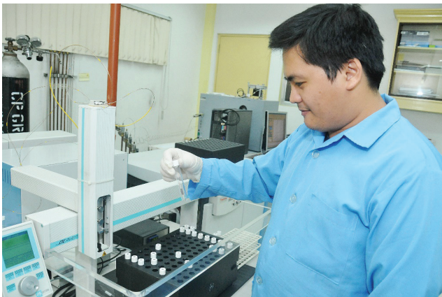
Water samples being analyzed with an isotope ratio-mass spectrometer to determine its characteristics
